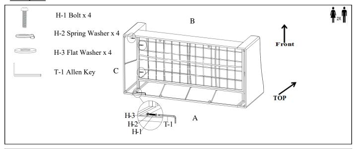
Secure the Left Arm (C) to the assembly with the Bolts (H-1), Spring Washers (H-2) and Flat Washers (H-3) using the provided Allen Key (T-1), staking the hardware in the order as shown. Engage all Bolts (H-1) first, then fully tighten. DO NOT OVER TIGHTEN.
