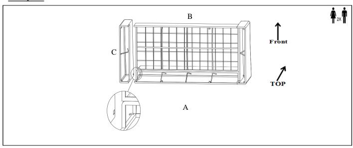
Position the Left Arm (C) with the Back Frame (A) as shown. Insert the metal hook on the Back Frame (A) into the hole in the top of the Left Arm (C) and engage.
