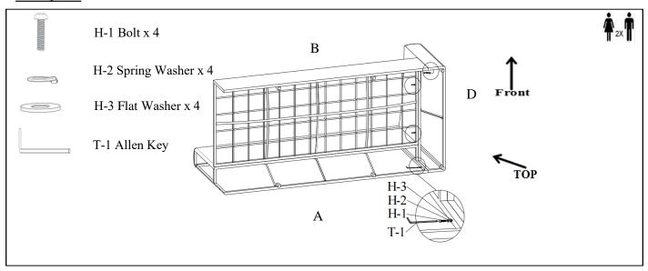
Secure the Right Arm (D) to the assembly with the Bolts (H-1), Spring Washers (H-2) and Flat Washers (H-3) using the provided Allen Key (T-1), staking the hardware in the order as shown. Engage all Bolts (H-1) first, then fully tighten. DO NOT OVER TIGHTEN.
