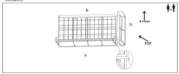
Position the Right Arm (D) with the Back Frame (A) as shown. Insert the metal hook on the Back Frame (A) into the hole in the top of the Right Arm (D) and engage.
