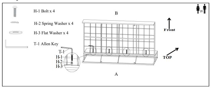
Carefully lay Back Frame (A) down onto a padded, non marring surface. Align holes in Seat Frame (B) with receiving holes in Back Frame (A) and secure all 2 mounting points with Allen Bolts (H-1), Spring Washers (H-2) and Flat Washers (H-3) using provided Allen Key (T-1), stacking the hardware in the order as shown. Engage all Bolts first then fully tighten. Do not over tighten.
